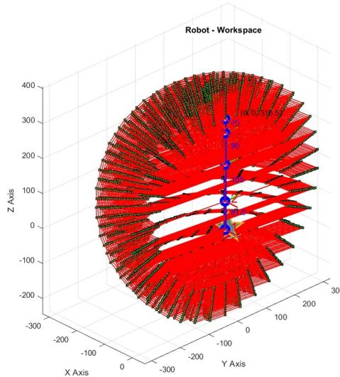
**Figure 5.** Robot working space in half-representation
