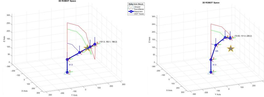
**Figure 3.** Robot positioning after using DKP in linear regression (left – using 2 parameters; right – using 4 parameters)
