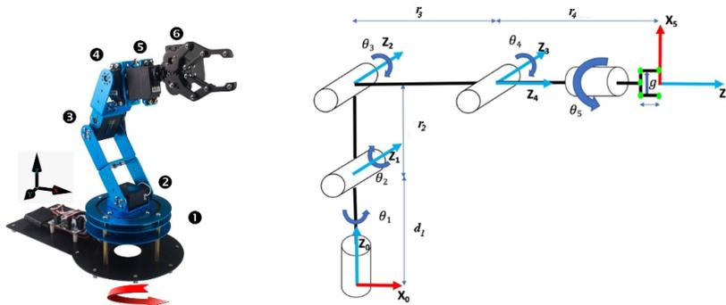
**Figure 1.** D-H Parameters of the testing robot (left – real model; right - virtual 3D model).
