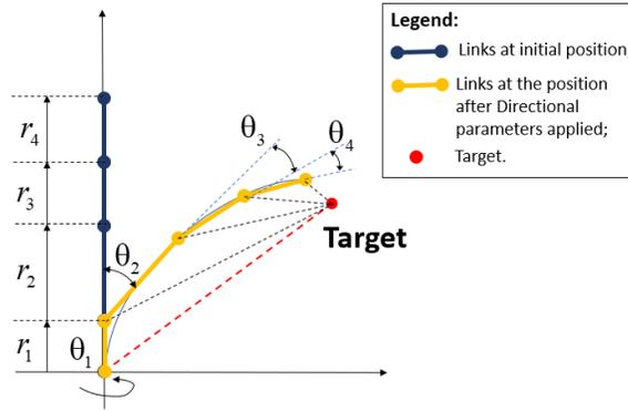
**Figure 2.** In plane D-H Parameters representation.
