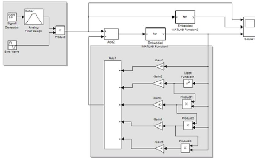
**Figure.2.** Matlab Simulink developed file to simulate the reduction of non-linearity of radiofrequency stages by introducing a feedback loop based on the reverse power series
