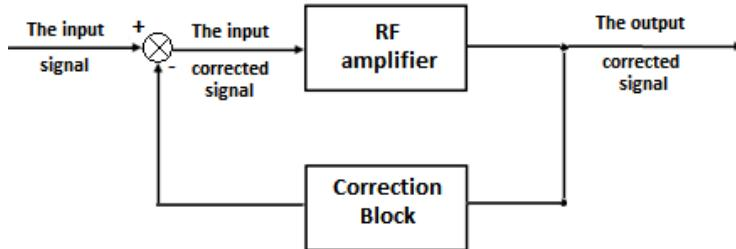
**Figure 1.** Compensate the operating effects of RF amplifiers in the nonlinear area by introducing a feedback loop
