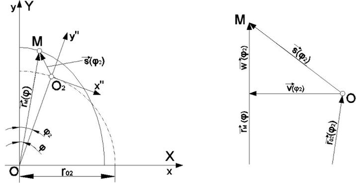
**Figure 2.** Positioning of a point M on the medium fiber of the deformed flexible wheel
