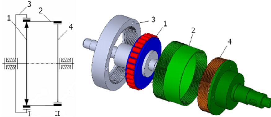
**Figure 1.** The scheme of the double harmonic transmission
