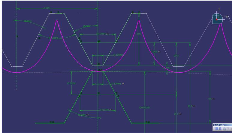
**Figure 5.** Trajectory of a point in the front section I of the flexible wheel
