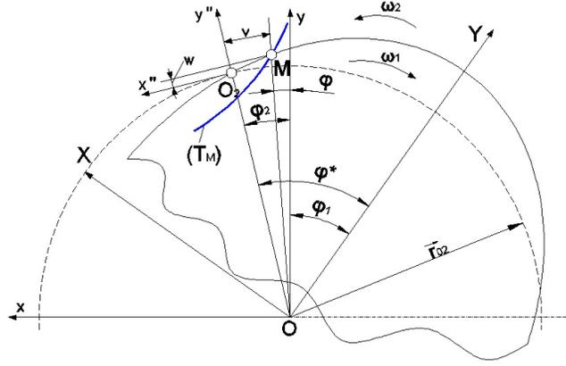
**Figure 3.** The trajectory of a point M on the average fiber of deformed flexible wheel
