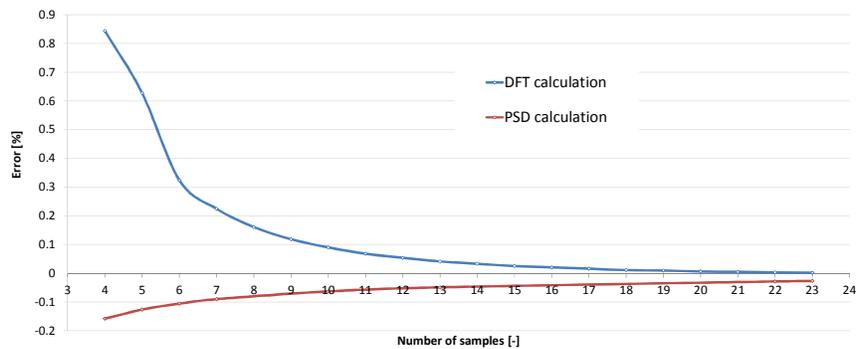
**Figure 4.** Error curves for interpolation made on DFT respectively PSD samples
