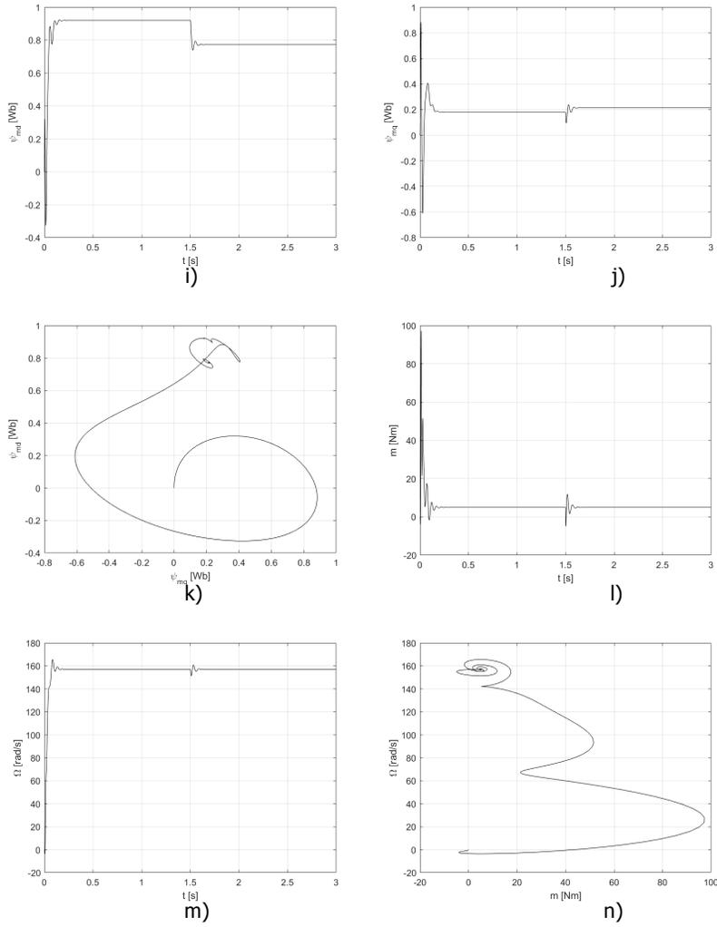
**Figure 2.** Characteristics obtained for:  $U=190$  V,  $J=0,01$  kgm<sup>2</sup>,  $M_r=5$  Nm.
