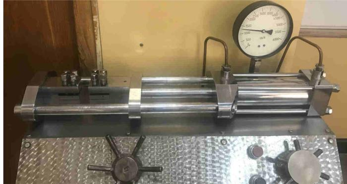
**Figure 1.** Hydraulic cylinder and tensile device.
