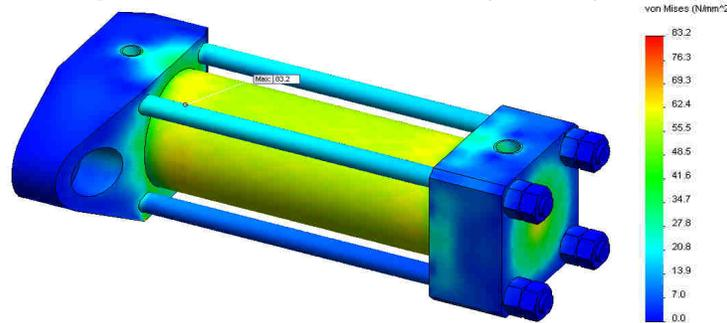
**Figure 4.** Von Mises stress distribution on cylinder.
