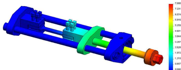
**Figure 10.** Resultant displacement distribution on tensile device.
