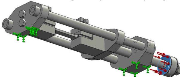
**Figure 7.** Loads and constraints on tensile device.
