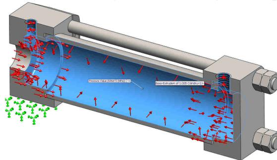
**Figure 3.** Loads and constraints on hydraulic cylinder
