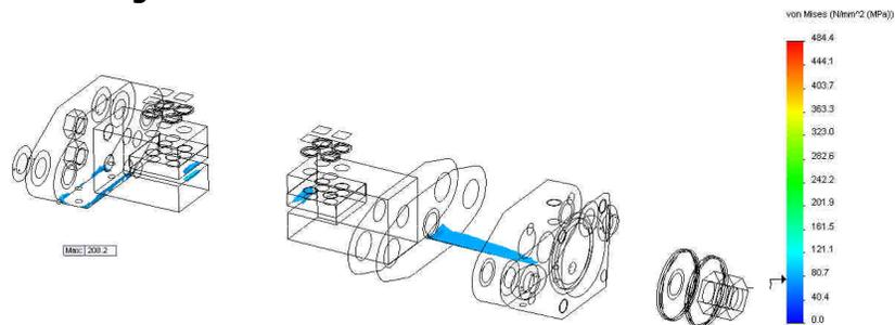
**Figure 9.** Tensile device. Area with von Mises stress above 75 N/mm<sup>2</sup>.
