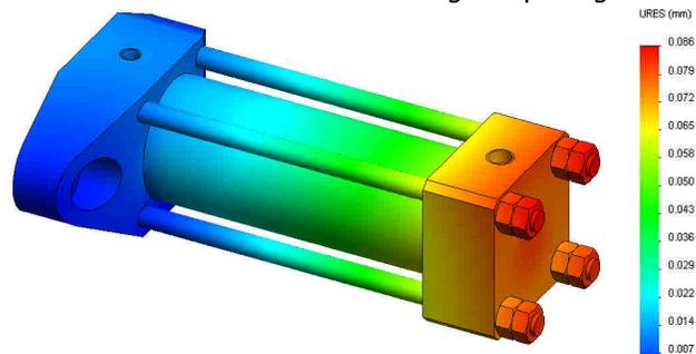
**Figure 6.** Resultant displacement chart on cylinder.
