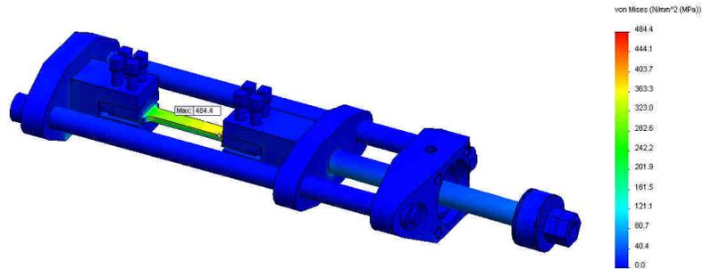
**Figure 8.** Von Mises stress distribution on tensile device.
