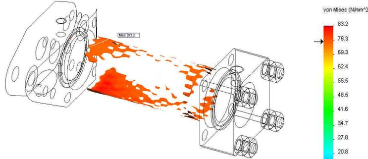
**Figure 5.** Area with von Mises stress above 75 N/mm<sup>2</sup>.
