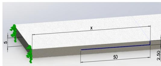
**Figure 10.** L-shaped crack - delamination oriented to the left
