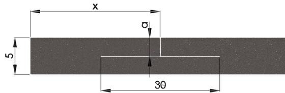
**Figure 8.** T-shaped crack.
