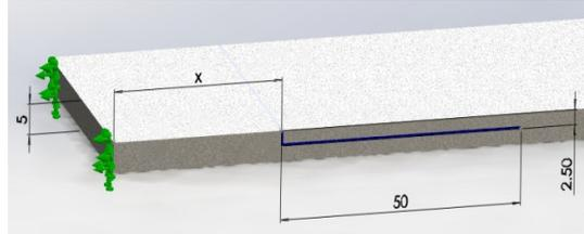
**Figure 11.** L-shaped crack - delamination oriented to the left right
