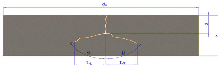
**Figure 7.** General dimensions of a maximum two branched crack.
