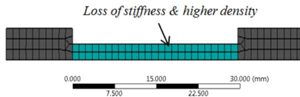
**Figure 4.** A zoom on the segment with a reduced thickness
