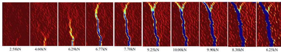
**Figure 3.** Crack propagation in reinforced concrete beams
