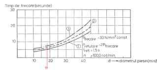
**Figure 1.** Determining the friction time depending on the thickness of the piece, [1]
