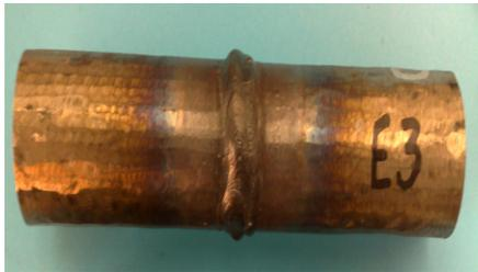
**Figure 1.** Point welded E3 sample, thermic untreated [1].
