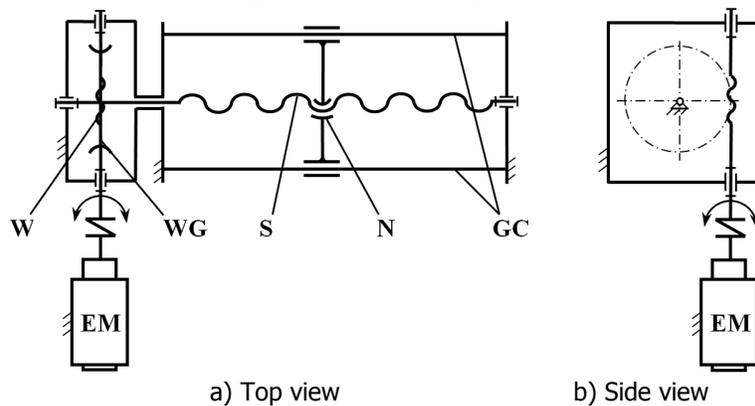
**Figure 2.** Kinematical scheme of the base mechanical transmissions [8]
