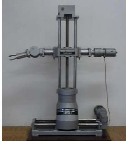
**Figure 1.** The 6-DOF industrial robot [7], [8], [11], [12]
