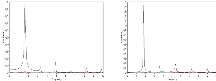
**Figure 6.** FFT of acceleration of top of the frame for steps from 0.5 to 5.5, black line - table, red line - frame.
