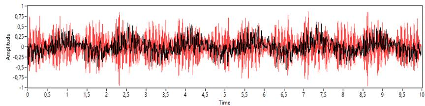
**Figure 5.** Acceleration [ $m/s^2$ ] of top of the frame (red line) and the table (black line) in time domain [s]
