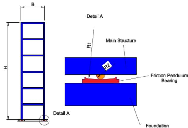
**Figure 3.** Friction pendulum bearing under the analyzed frame.
