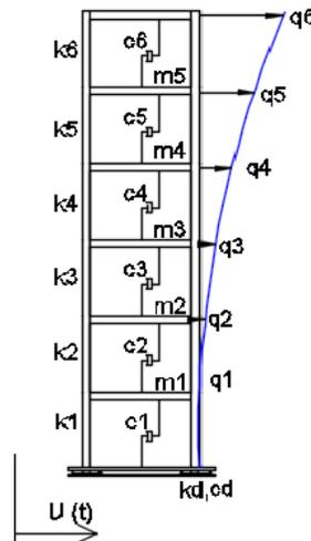
Figure 1. Model of the frame with Friction Pendulum Bearings
