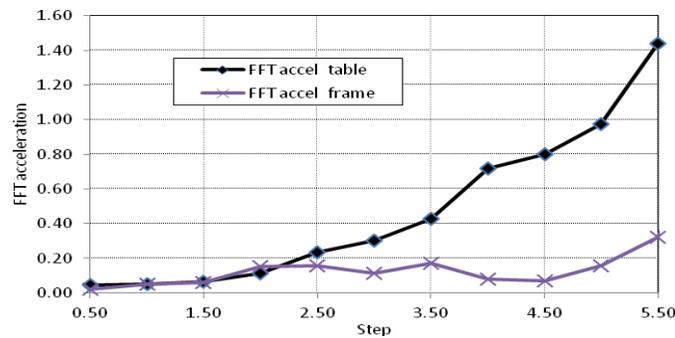
**Figure 7.** FFT of acceleration of top of the frame for steps 0.5 to 6.0, black line - table, red line - frame.
