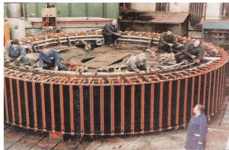
**Figure 21** The bulb generator rotor
