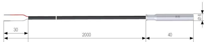
**Figure 5.** The PT 1000 temperature sensor.
