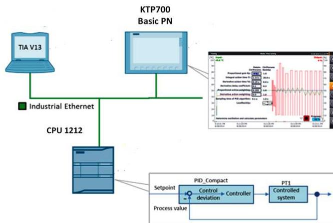
**Figure 1.** Highlighting the components of the control system with PLC S7-1200 by using the logical function "PID\_Compact"
