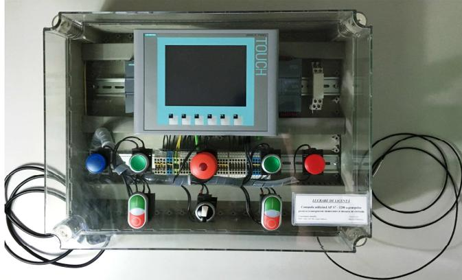
**Figure 7.** The box which contains the TOUCH panel.
