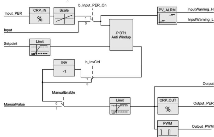
**Figure 2.** PID\_Compact – the block diagram
