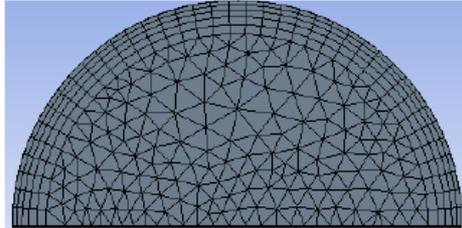
**Figure 9.** Mesh distribution of the duct
