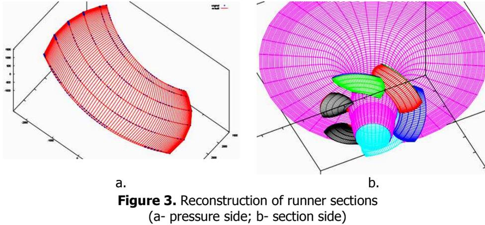
Further, QTurbo3D plots the re-built blade, using the library of Gnuplot distribution. Also, the presence of hub surface helps the user to better understand the shape and orientation of the runner blades in the assembly.
