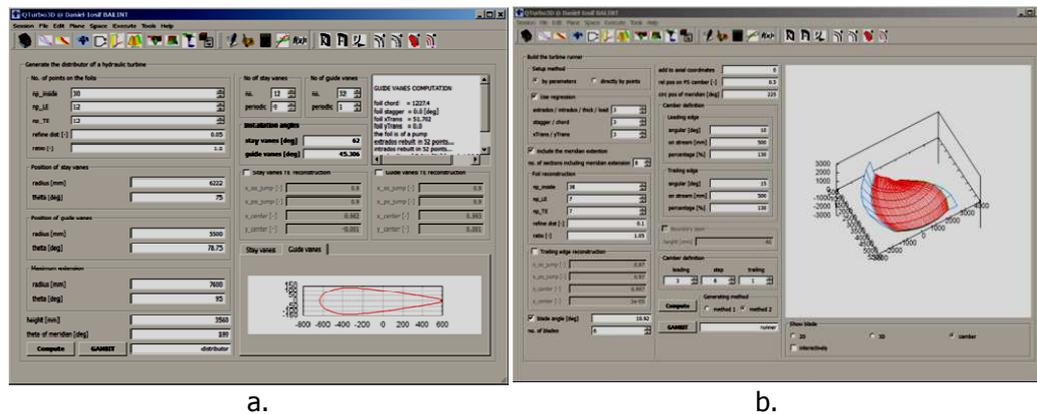
The computation of the flow is performed using Fluent/ANSYS distribution, while the geometry is built in Gambit pre-processor of Fluent package. QTurbo3D generates the scripting files for building automatically the computation domains as presented in Figure 4 a. for the guide vane and Figure 4 b for the runner domain.
