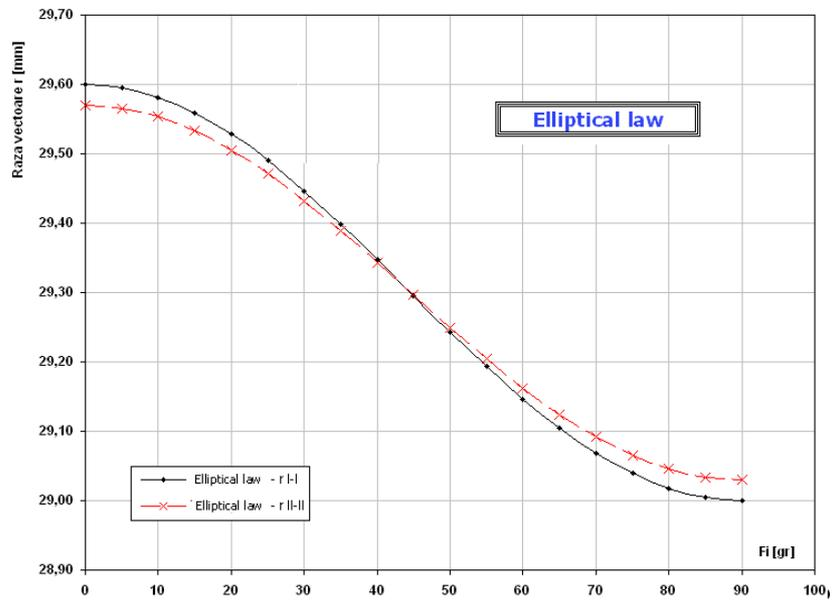
**Figure 4.** Diagrams of vector rays of deformed flexible wheel - elliptical law
