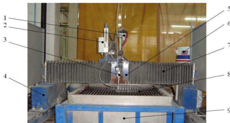
Figure 2. Water jet cutting equipment
