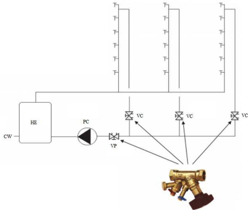
**Figure 3.** DHW plumbing installation with recirculation, heat exchanger, recirculation pump, balancing valves on columns and Partner valve [2]
