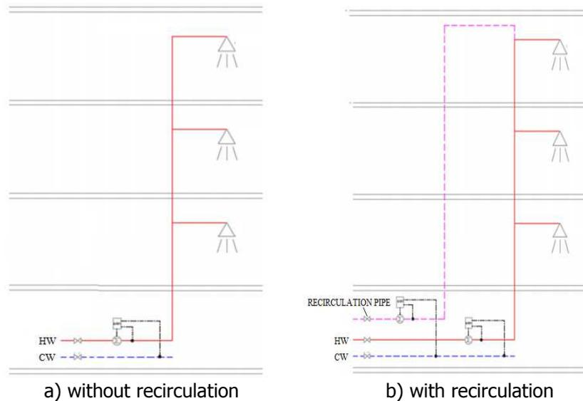
**Figure 1.** Plumbing installation for domestic hot water supply
