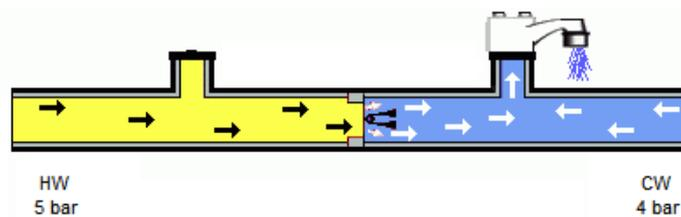
**Figure 8.** Cold water siphon phenomenon [15]
