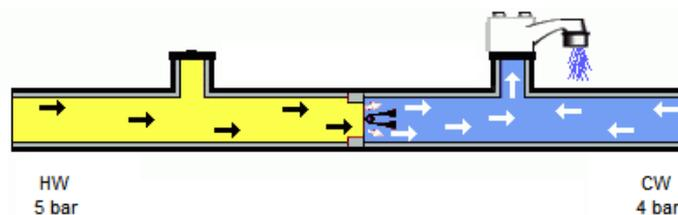
**Figure 8.** Cold water siphon phenomenon [15]
