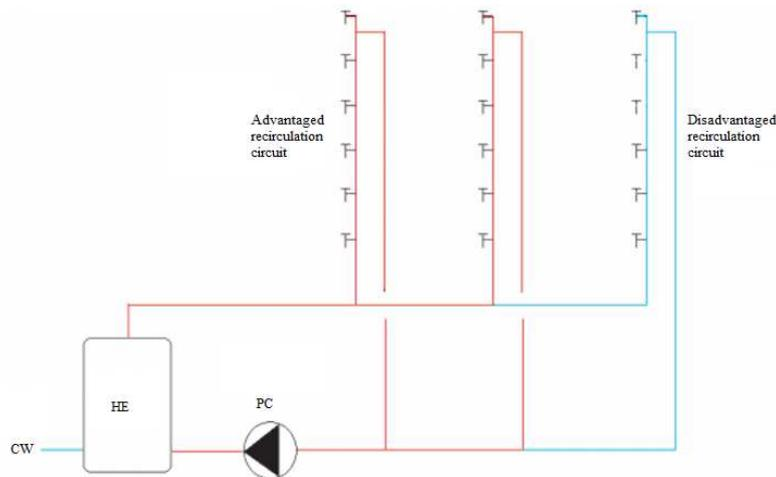
**Figure 2.** DHW plumbing installation with recirculation, heat exchanger and recirculation pump [2]
