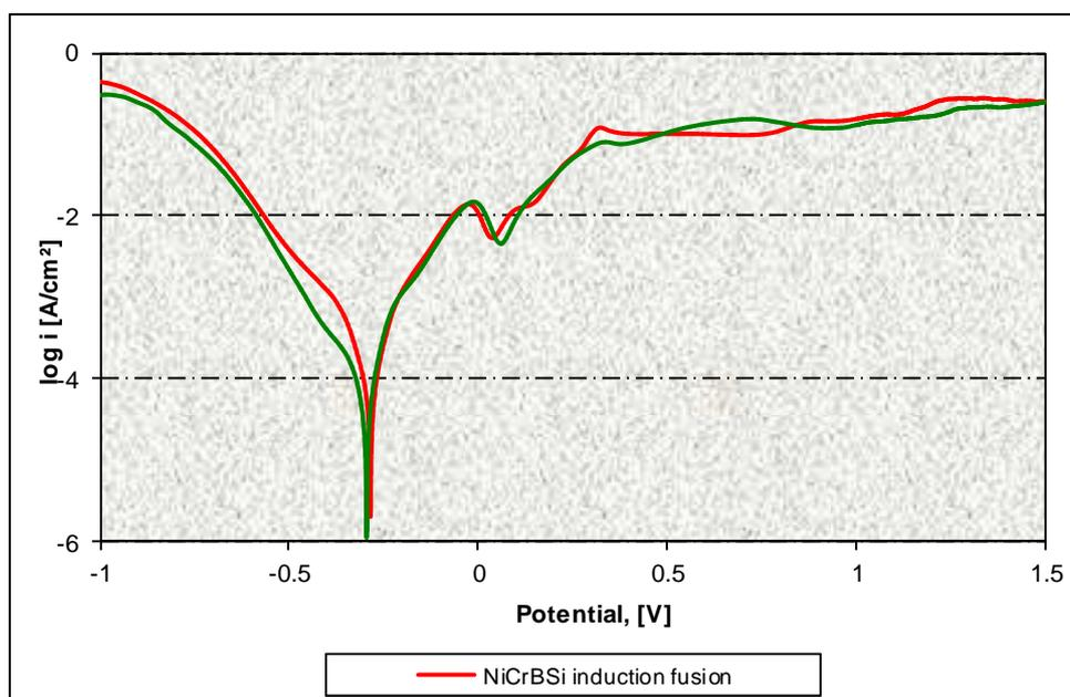
**Figure 4.** Potentiodynamic polarization curves of the samples tested in a 3,5% NaCl solution
