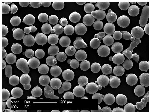
**Figure 1.** SEM-micrograph of the NiCrBSi powder
