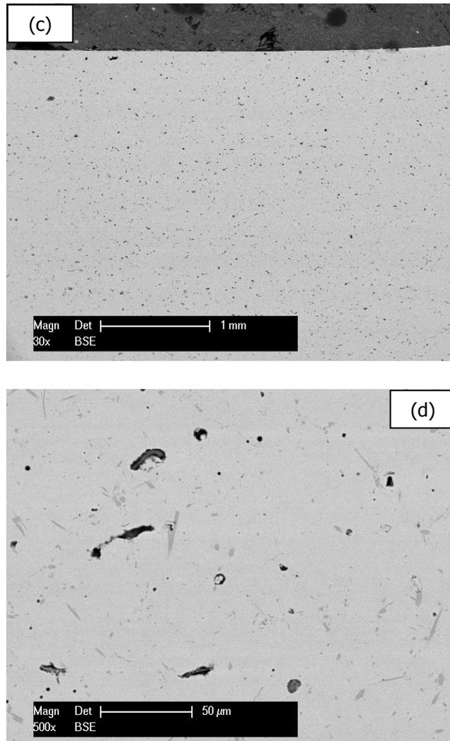
**Figure 2.** Cross-section SEM-micrographs of the fused coatings: induction (a, b) and oxy-acetylene flame (c, d)
