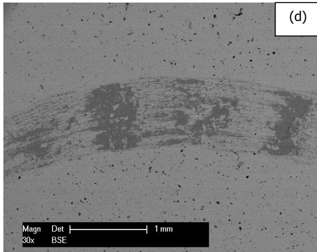
**Figure 6.** SEM-micrographs of the worn surface of the induction fused coating (a, b) respectively of the flame fused coating (c, d)
