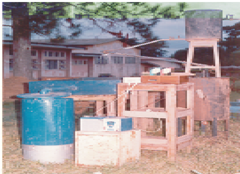
Figure 2. Automatic Runoff-meter during operation at gradient 5^\circ .
