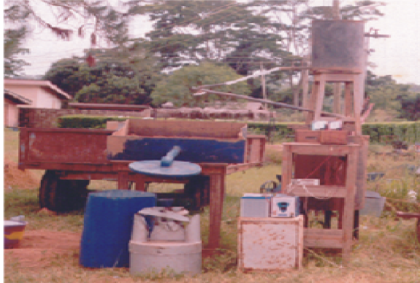
Figure 3. Automatic Runoff-meter disassembled after operation
