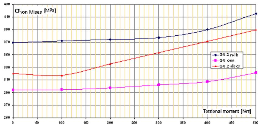
**Figure 4.** Maximum von Mises stress diagram,  $\sigma_{VM} = \sigma_{VM}(M_{t4})$
