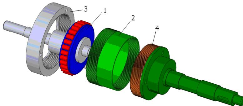
**Figure 1.** The scheme of a double harmonic gear transmission.
