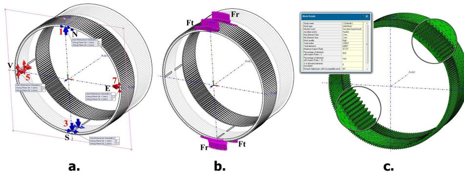
**Figure 3.** Restrictions applied to the tasks and meshing to the flexible wheel.
