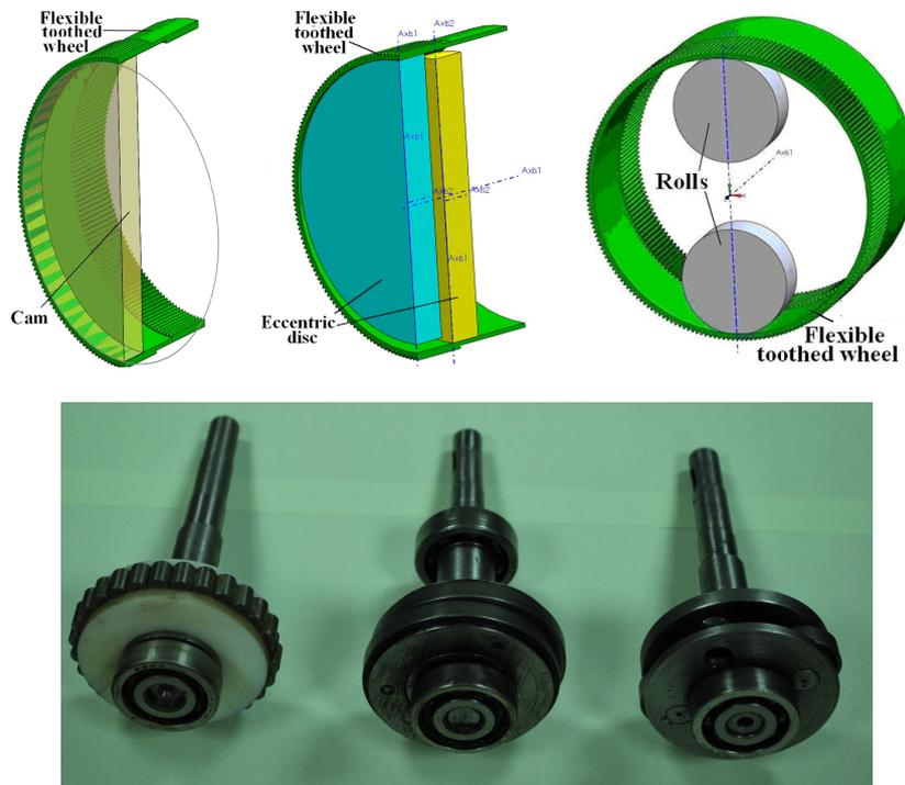
**Figure 2.** The models of a waves generator.
