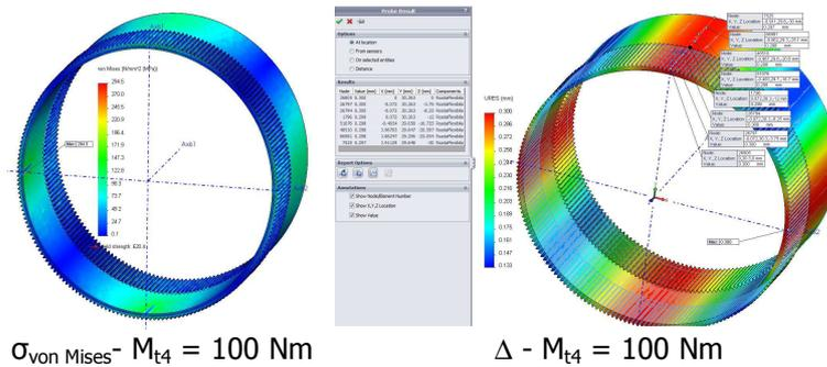
**Figure 6.** The von Mises stress ( $\sigma_{vMmax}$ ) and the resultant displacement ( $\Delta$ ).
