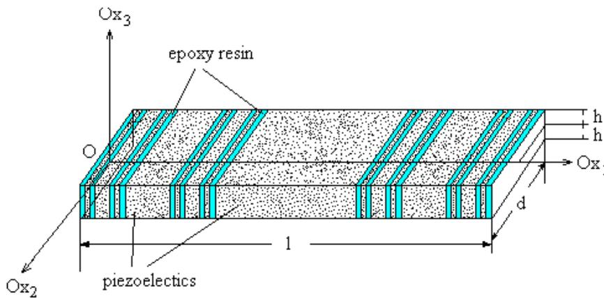
**Figure 4.** The non-periodic structure with Cantor-like structure
