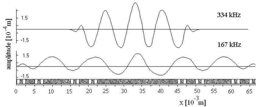
**Figure 5.** Lamb displacement of the normal and subharmonic modes
