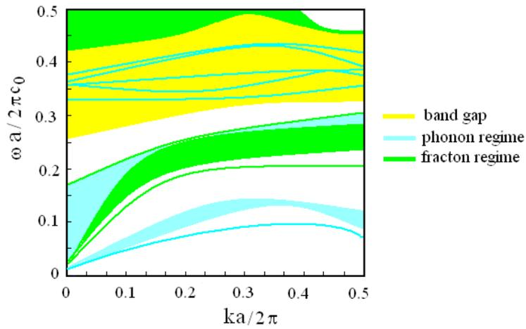
**Figure 8.** Lamb band structure
