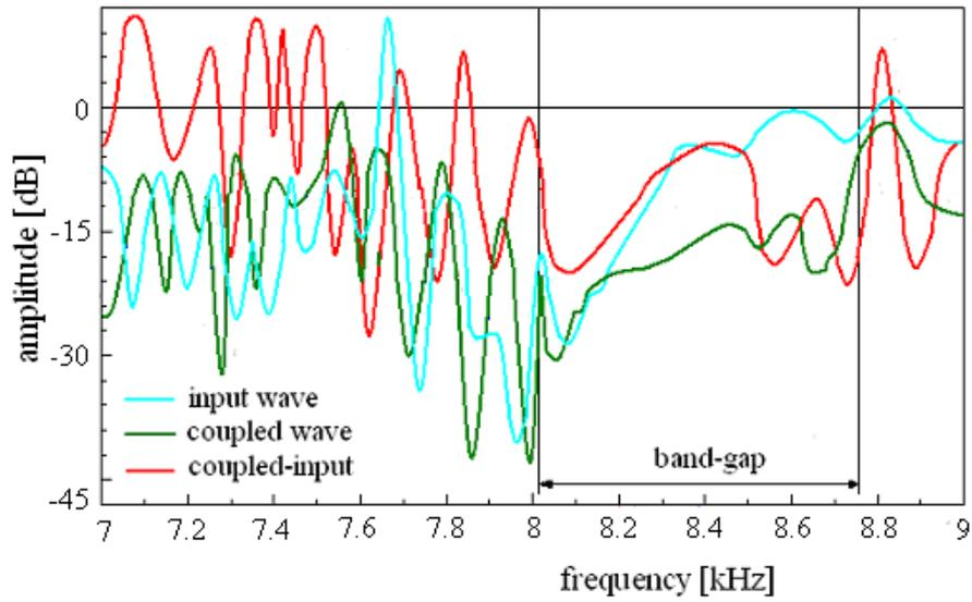
**Figure 1.** The input and coupled waves for the sonic composite
