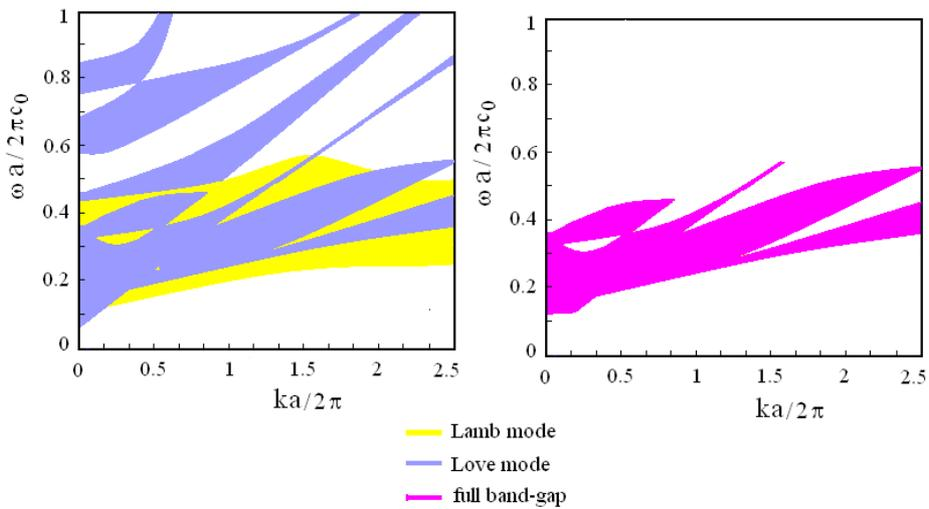
**Figure 9.** Love band structure (left) and the full band-gap (right)
