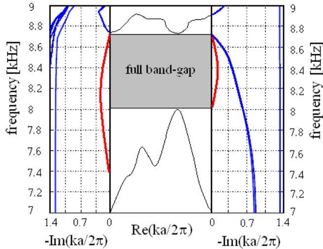
**Figure 3.** Band structure for the sonic composite
