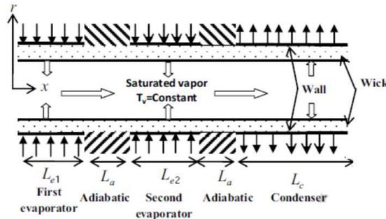
**Figure 3.** Schematic of a cylindrical heat pipe with two evaporators [26]
