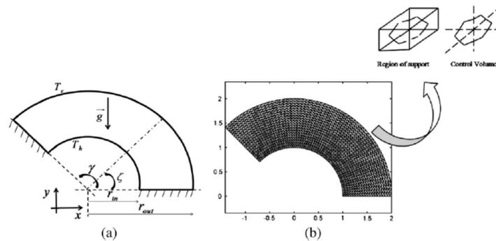
**Figure 5.** (a) Geometry and the boundary conditions with (b) the mesh of semi-annulus enclosure considered in this work. [39]
