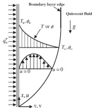
**Figure 4.** Vertical plate with a constant surface heat flux [33]
