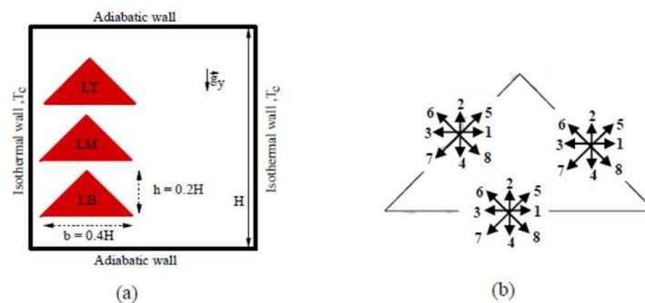
**Figure1.** (a) Sketch of studied configuration and (b) Lattices positions at the triangle faces for the D2Q9 arrangements [14]
