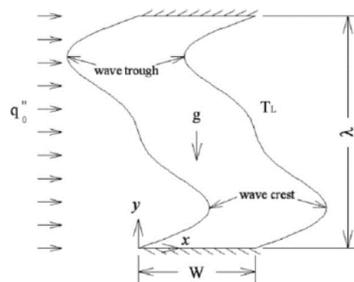
**Figure 2.** Schematic illustration of wavy-wall enclosure. Note that  $g$  indicates the gravitational acceleration [20]
