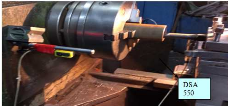
Figure 3. Speedometer fixing with Doppler effect, with multilane laser with magnetic support.
