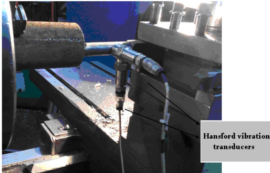
Figure 4. Accelerometer fixing with magnetic support.
