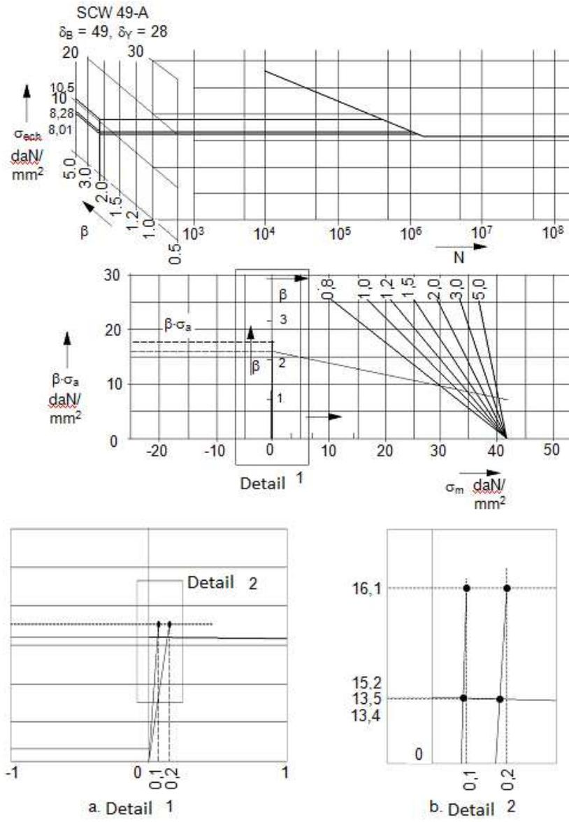
**Figure 3.** Fatigue diagram from rotating bending stress [3]
