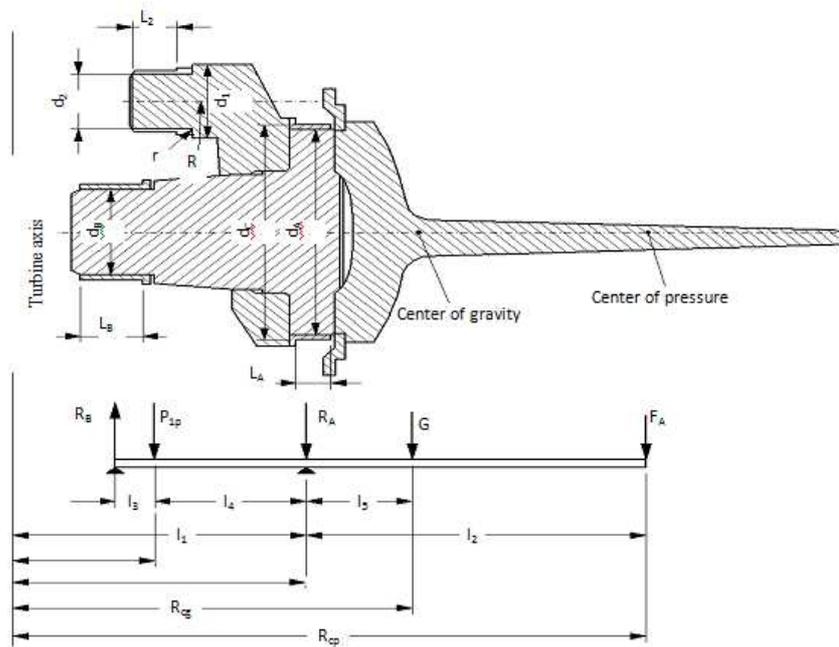
**Figure 2.** Load diagram of blade spindle
