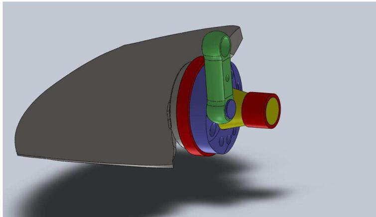
**Figure 1.** Runner blade – operating mechanism assembly.
