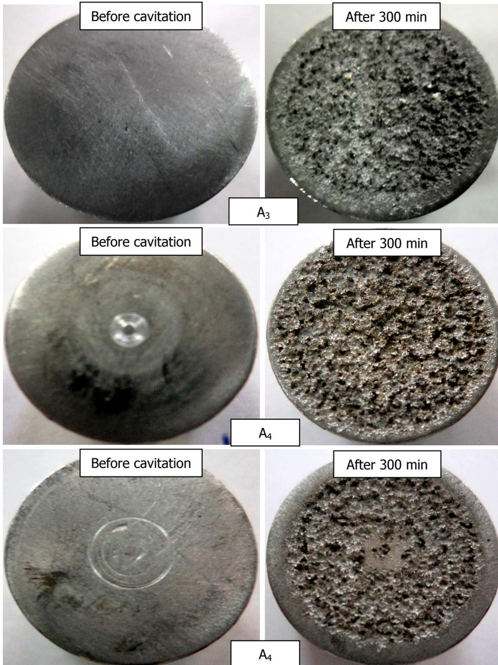
**Figure 5.** The appearance of surfaces before and after total time of exposure to cavitation
