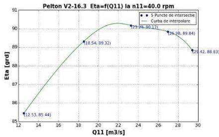
**Figure 13.**  $\eta = f(Q_{11})$  2D curve for  $n_{11}=40.0$  rpm - V2-16.3 Pelton runner
