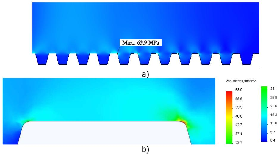
**Figure 4.** Von Mises stress variation for the bolt with R=0.6 mm: a) overview and b) details on the root area of the first thread turn of bolt – nut interface
