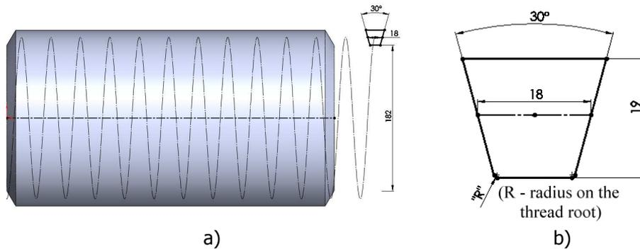
**Figure 1.** Main parameters of threaded bolt
