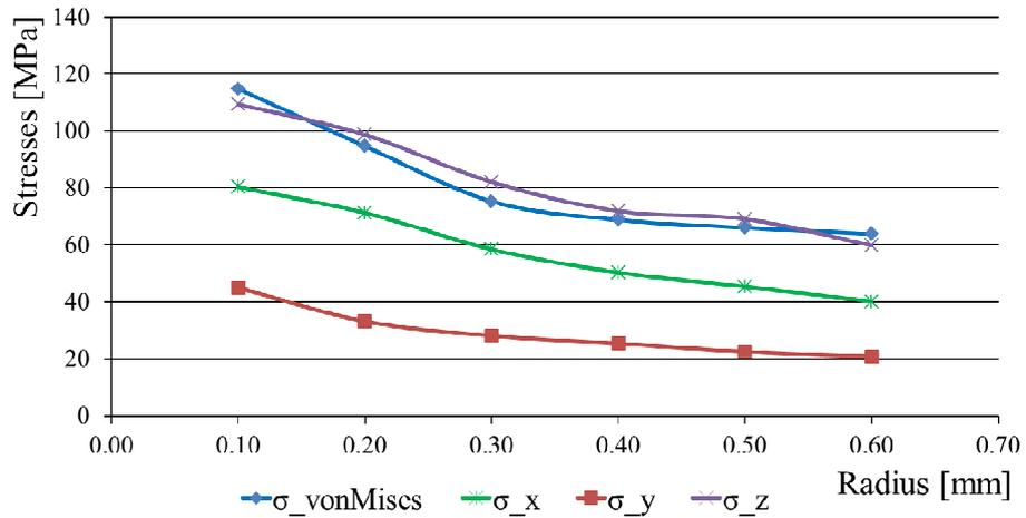
**Figure 3.** Stresses vs. thread root radius variation
