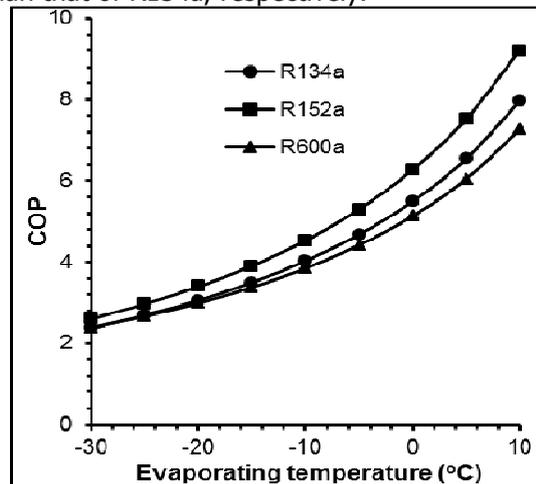
**Figure 7.** Coefficient of performance (COP) versus evaporating temperature at condensing temperature of 40°C.
