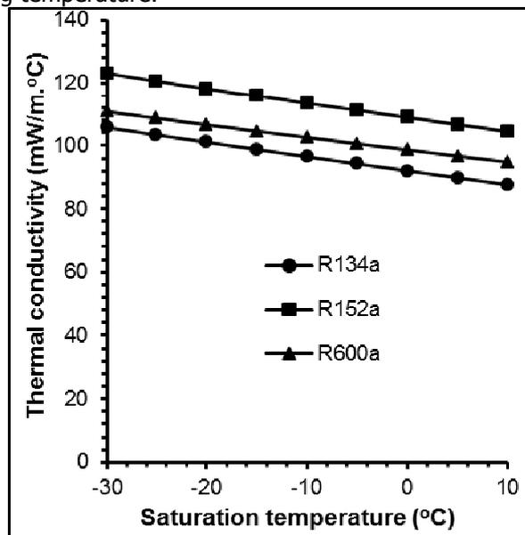
**Figure 4.** Variation of thermal conductivity with saturation temperature
