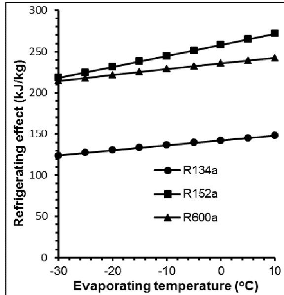
**Figure 5.** Variation of refrigerating effect with evaporating temperature at condensing temperature of 40°C.
