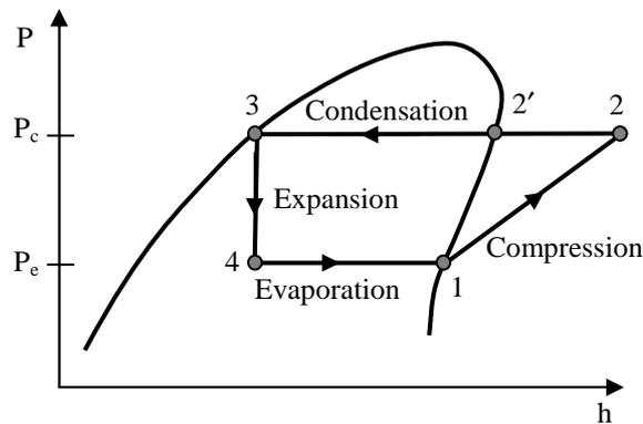
Figure 1: vapour compression refrigeration cycle on p-h diagram
