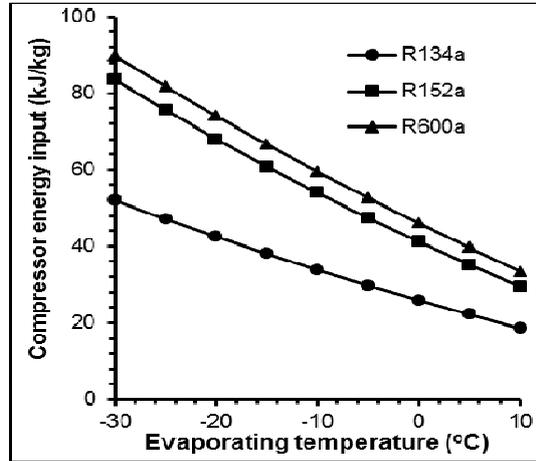
**Figure 6.** Variation of compressor energy input with evaporating temperature at condensing temperature of 40°C.
