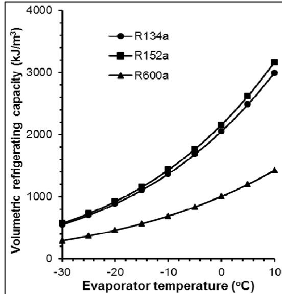
**Figure 9.** Influence of evaporator temperature on the volumetric refrigerating capacity at condensing temperature of 40°C
