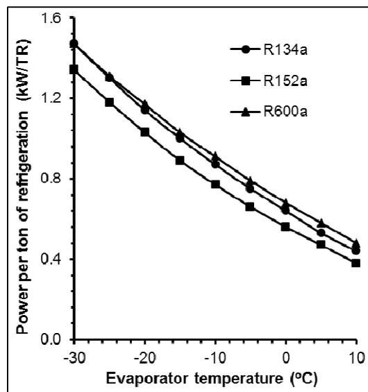
**Figure 8.** Influence of evaporating temperature on the power per ton of refrigeration at condensing temperature of 40°C
