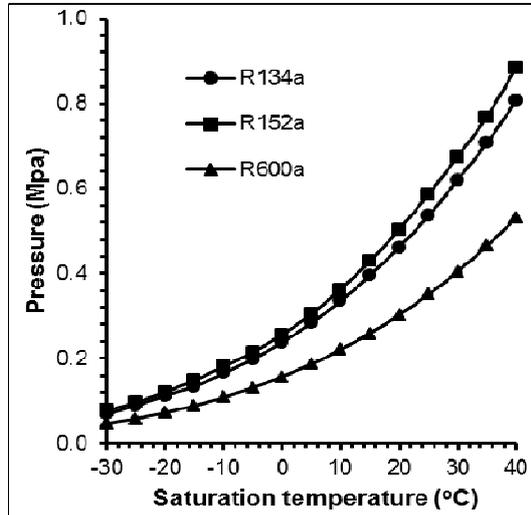
**Figure 2.** Saturation pressure and temperature curves
