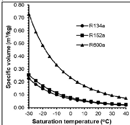
**Figure 3.** Specific volume of refrigerant vapour versus saturation temperature
