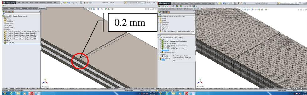
**Figure 1.** Portion of defective rod and the mesh mode for beam with 1x0.2 mm damage dimension
