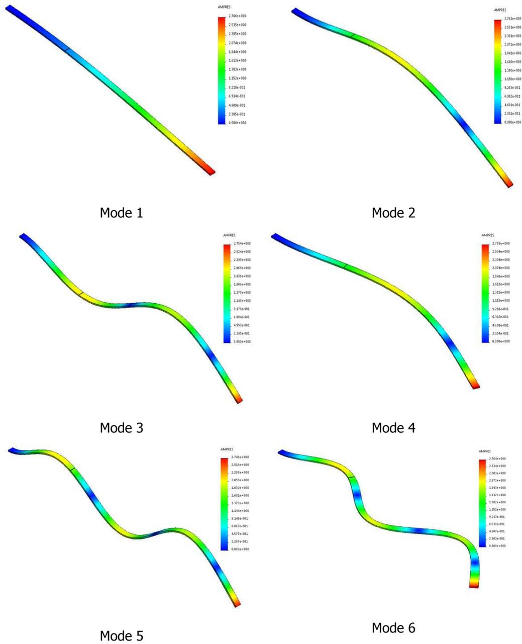
**Figure 4.** First six vibration modes for damaged beam
