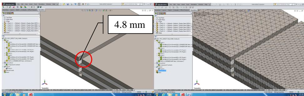
**Figure 3.** Portion of defective rod and the mesh mode for beam with 1x4.8 mm damage dimension
