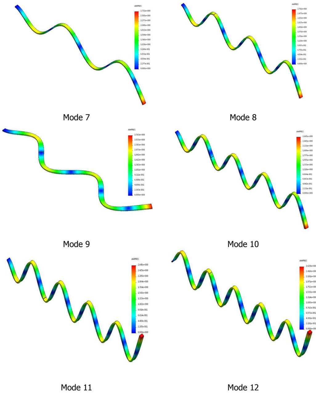
**Figure 5.** Vibration modes seven to twelve for damaged beam
