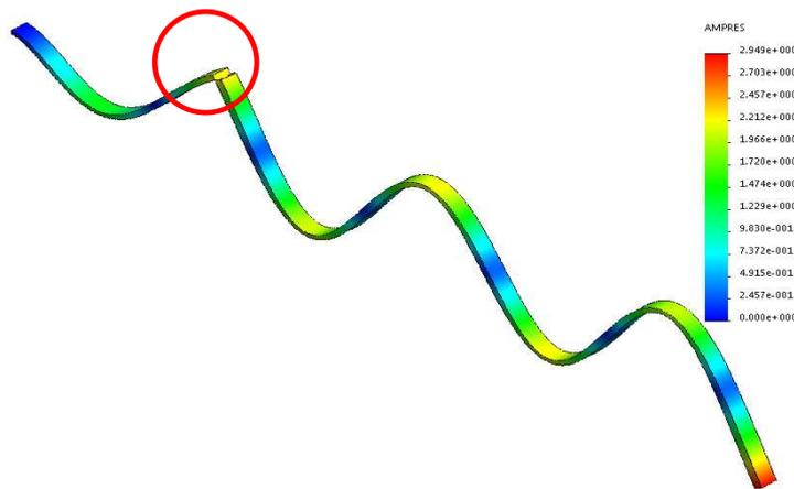
**Figure 7.** Eighth vibration mode shape of the beam with defect at  $x / L = 0.274$  m
