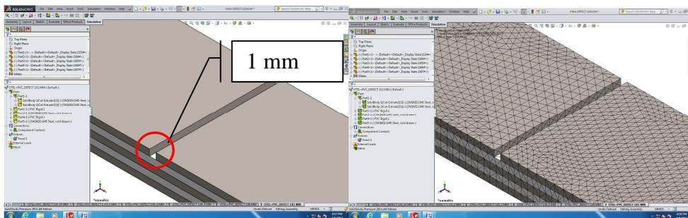
**Figure 2.** Portion of defective rod and the mesh mode for beam with 1x1 mm damage dimension
