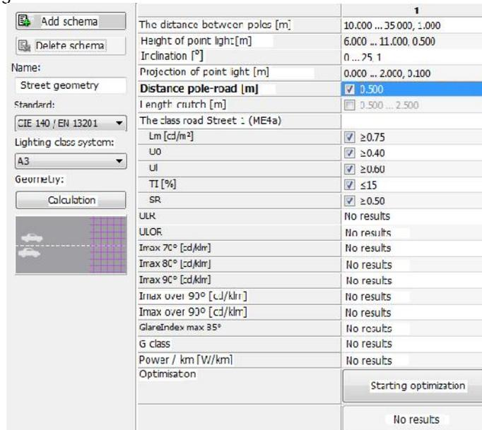
Figure 4. Setting measure ranges for the indicators to be optimized.
