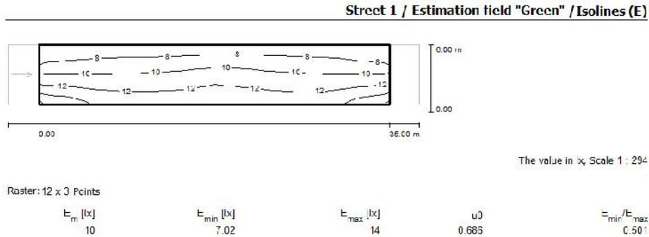
Figure 3. Lighting indicator values and isolux curves.
