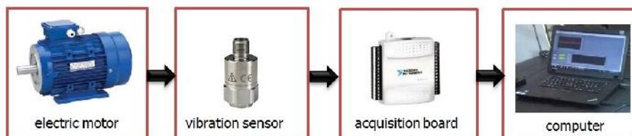
Figure 1. Block diagram system for acquisition, monitoring and vibration analysis.
