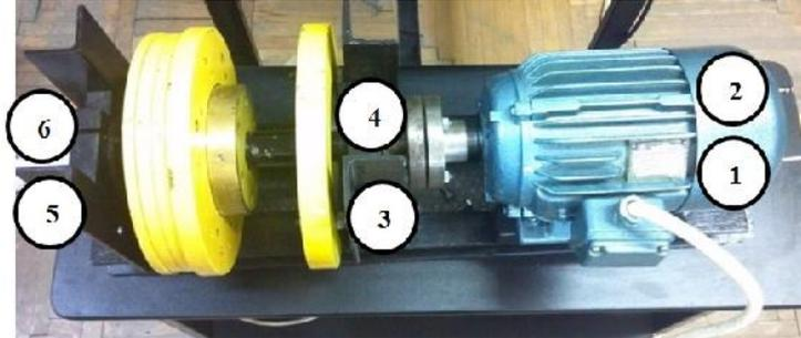
Figure 3. Vibrations measurement points.
