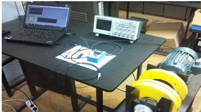
Figure 2. Experimental arrangement for acquisition, monitoring and vibration analysis at an induction motor.
