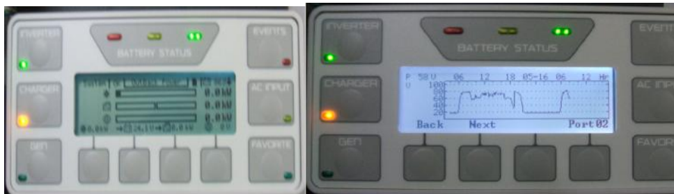
Figure 8. Photovoltaic system parameters display: a) numeric display; b) graph display
