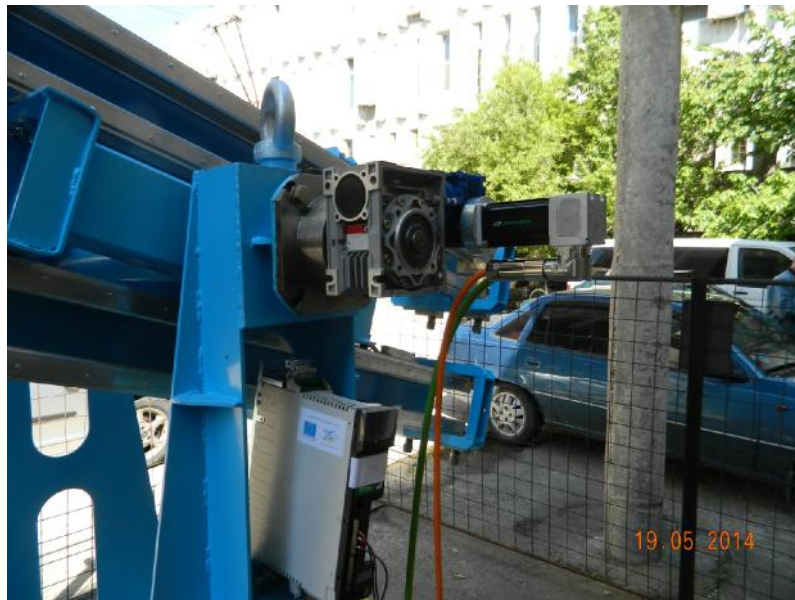
Figure 6. Elevation drive mounted on the ramp.
