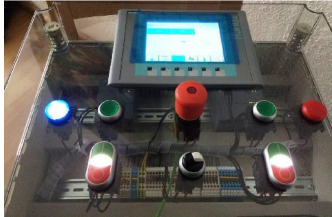
Figure 8. Frontal panel: Simulating the functioning of a pump at minimum pressure
