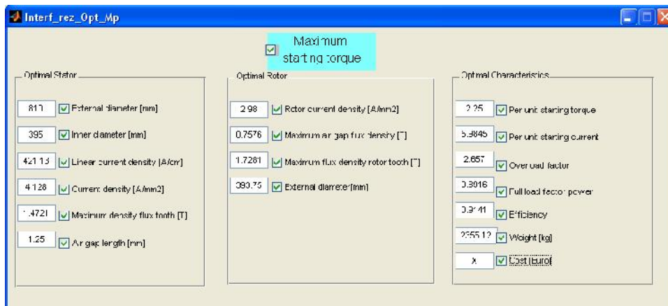
Figure 7. The optimal design parameters - the optimization criterion: maximum starting torque.
