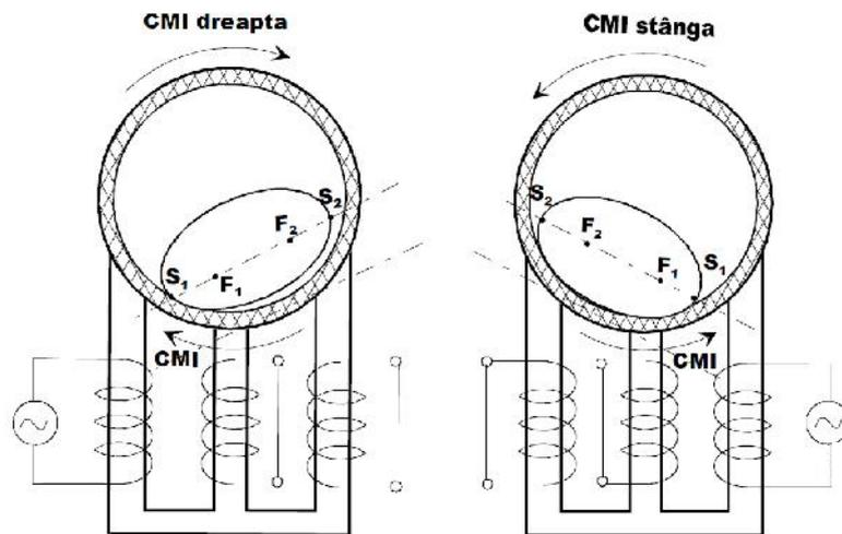
Figure 6. GROSU-CERNOMAZU motor. The ferrofluid movement spectrum has the shape of a distorted ellipse, with the major axis oriented in the shielded pole direction [15].
