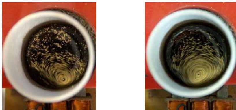
Figure 7. The movement spectrum for the use of a magnetoactive particles slurry for GROSU – CERNOMAZU motor, according to the phase sequence [15]: a). Direct sequence (R-S-T); b). Reverse sequence (T-S-R)
