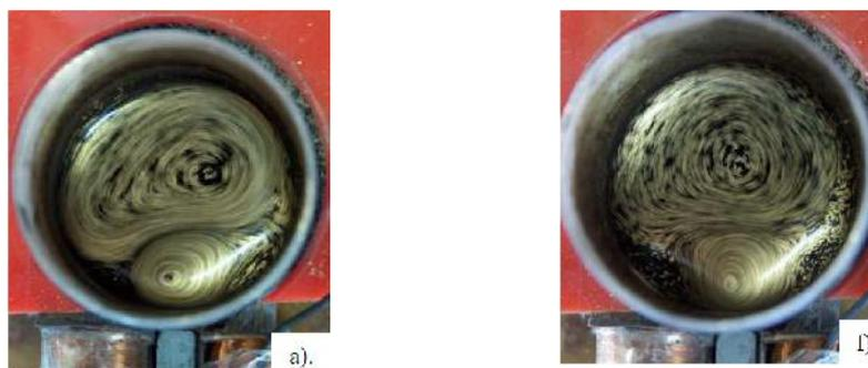
Figure 9. The movement spectrum for the use of a magnetoactive particles slurry, for a GROSU three-phase motor with “V” connection [15]: a). Direct sequence (R-S-T); b). Reverse sequence (T-S-R).
