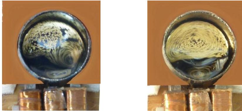
Figure 10. The movement spectrum for the use of a real ferrofluid, for a GROSU three-phase motor with "V" connection:
