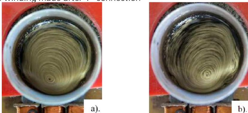
Figure 4. The movement spectrum for the use of a magnetoactive particles slurry, according to the phase sequence [42]: a). Direct sequence (R-S-T); b). Reverse sequence (T-S-R).
