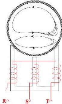
Figure 11. Explanatory at the forming of ferrofluid movement spectrum exposed to the rotating magnetic field action produced by a three – phase GROSU fixed coil with „V” connection supplied by a three-phase source 3X380 V; 50 Hz [15].
