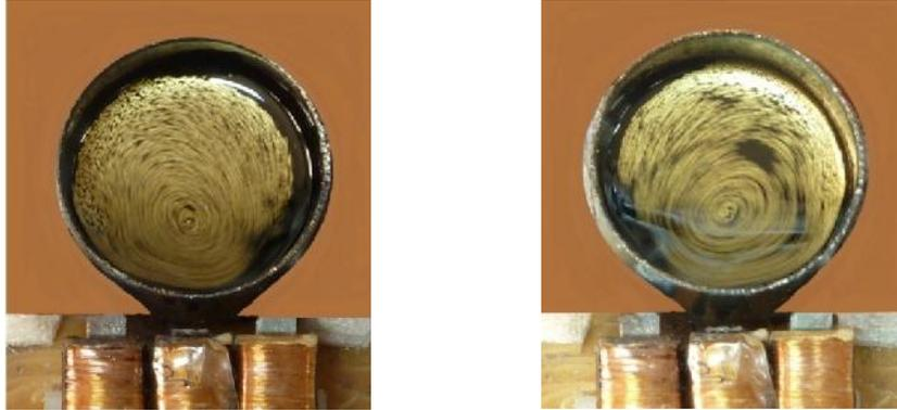
Figure 5. The movement spectrum for the use of a real ferrofluid, according to the phase sequence: a). Direct sequence (R-S-T); b). Reverse sequence (T-S-R).
