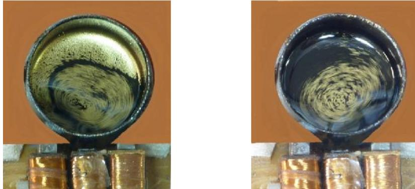
Figure 8. The movement spectrum for the use of a real ferrofluid for GROSU – CERNOMAZU motor, according to the phase sequence: a). Direct sequence (R-S-T); b). Reverse sequence (T-S-R)
