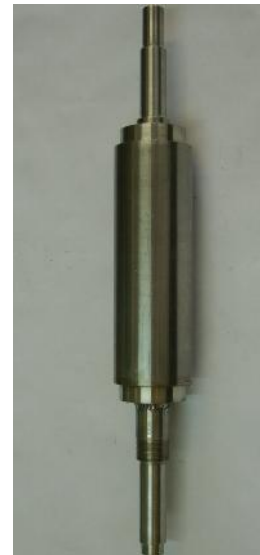
Figure 14. Rotor of hermetic asynchronous motor with stainless steel cylinders serially produced
