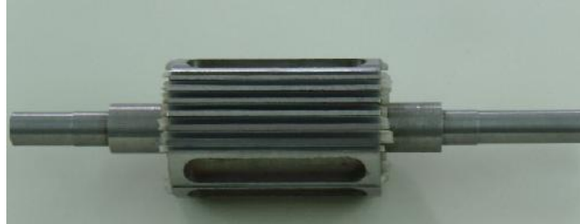
Figure 15. Rotor of synchronous motor made of ferromagnetic material
