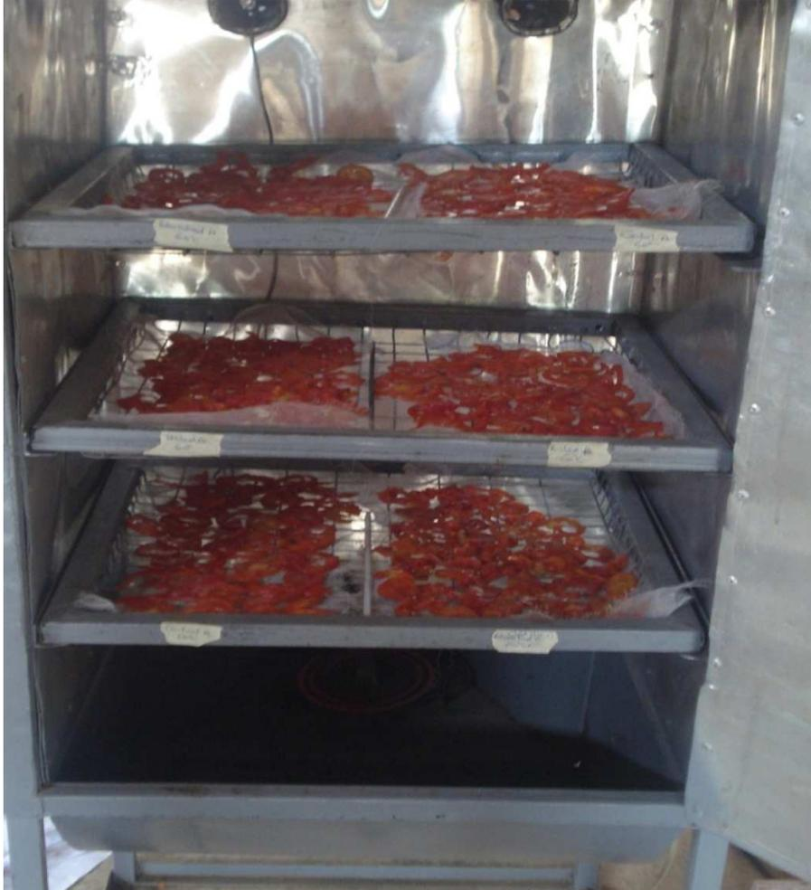
**Figure 3.** Arrangement of tomatoes on the trays in the dryer
