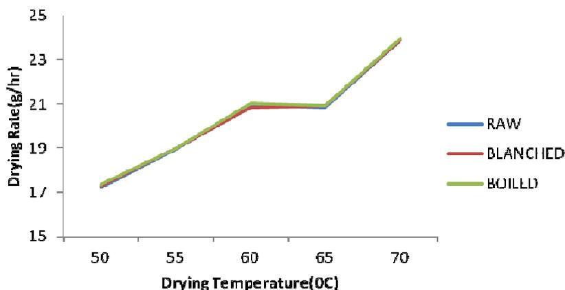
**Figure 5.** Effect of Pre-treatment on Drying Rate at different Drying Temperature
