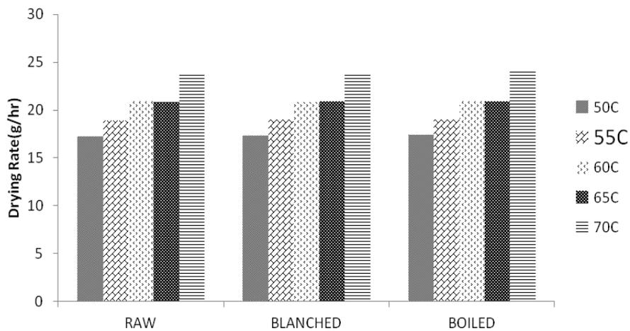
**Figure 4.** Effect of Pre-Treatment on Drying Rate at different Drying Temperature
