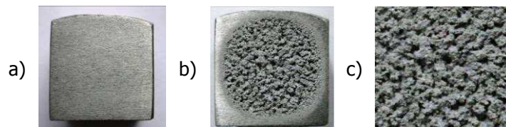
Figure 13. Surface images before cavitation a), after cavitation b) and the macrostructure of eroded surface c), for time periods of 30 minutes.
