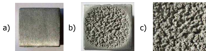
Figure 12. Surface images before cavitation a), after cavitation b) and the macrostructure of eroded surface c), for time periods of 15 minutes.
