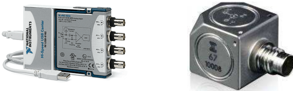
Figure 10. Experimental stand for modal analysis of damaged plate with NI USB-9233 acquisition system and tri-axial accelerometer
