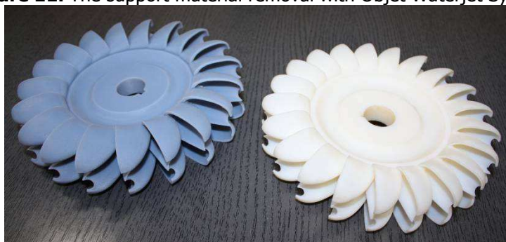
Figure 12. The final shape of the two Pelton runners (The runner V1 with 19 bucket and the runner V2 with 21 bucket)
