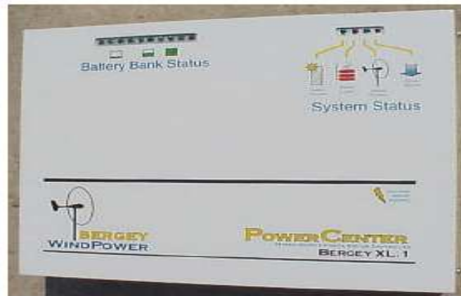
Figure 3. The Power Center Controller for BWC XL.1
