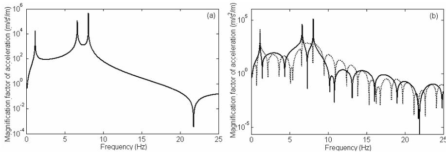
**Figure 6.** The magnification factors of the vertical acceleration: (a) non-filtered; (b) filtered,  $\cdots$ ,  $V = 100$  km/h;  $\text{—}$ ,  $V = 200$  km/h.
