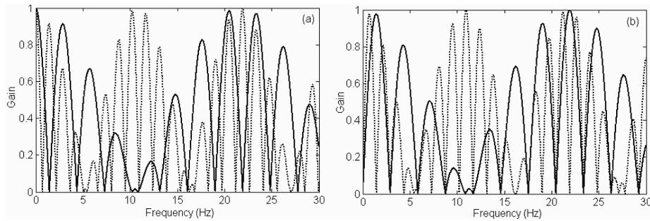
**Figure 3.** Influence of velocity upon the frequency characteristics of the vehicle excitation modes: (a) symmetrical mode; (b) skew-symmetrical mode:  $\cdots$ ,  $V = 100$  km/h; —,  $V = 200$  km/h.
