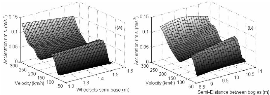
**Figure 9.** The r.m.s. acceleration in the center of carbody:
