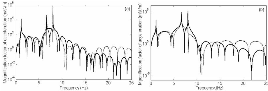
**Figure 8.** Influence of carbody axle base upon the magnification factor of vertical acceleration: (a)  $V = 100$  km/h; (b)  $V = 200$  km/h:
