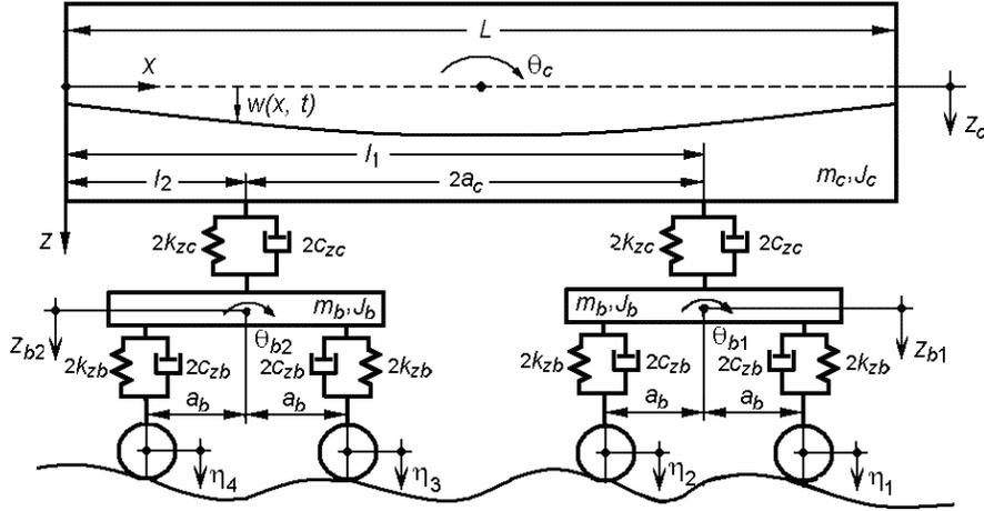
**Figure 1.** The vehicle mechanical model.
