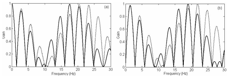
**Figure 4.** Influence of bogie axle upon the frequency characteristics of vehicle excitation modes: (a) symmetrical; (b) skew-symmetrical:
