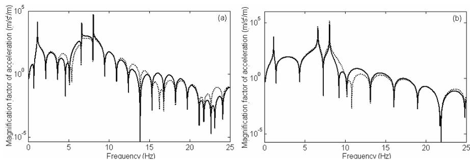
**Figure 7.** Influence of bogie axle base upon magnification factor of the vertical acceleration: (a)  $V = 100$  km/h; (b)  $V = 200$  km/h:
