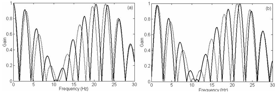
**Figure 5.** Influence of carbody axle base upon the frequency characteristics of the vehicle excitation modes: (a) symmetrical; (b) skew-symmetrical:  $\cdots$ ,  $2a_c = 17$  m;  $\text{—}$ ,  $2a_c = 19$  m.
