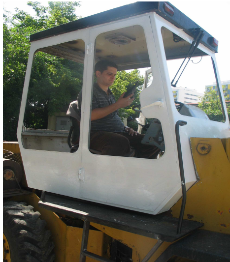
Figure 3. Determining the level of noise in the cabin of MMT45, in charge (without acoustic treatment)
