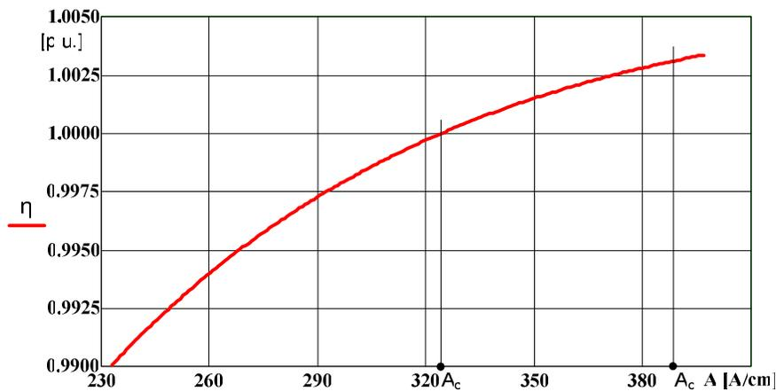
**Figure 4.** Efficiency variation curve depending on the current layer
