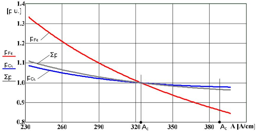
**Figure 3.** Loss variation curves depending on the current layer for a synchronous generator
