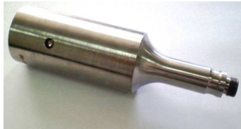
Figure 2. Sonotrode with M12x1 external thread used for direct method
