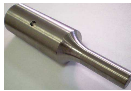
Figure 3. Sonotrode without thread used for indirect method
