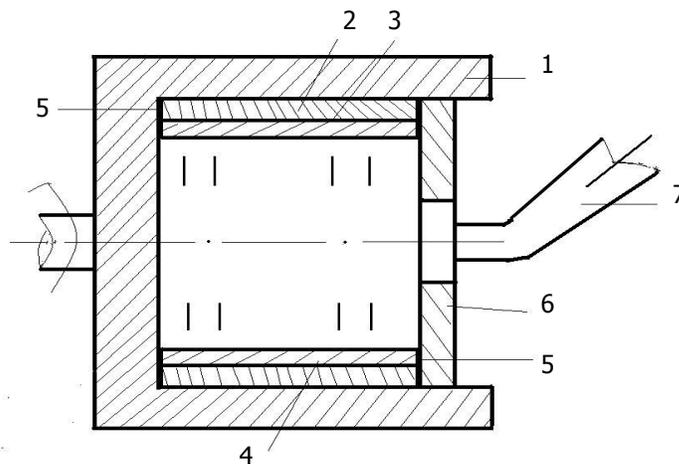
**Figure 2.** The scheme of centrifugal casting installation for bimetalllic bearings: 1 - machine housing; 2 - steel support; 3 - metallic layer of adhesion (tin), 4 - layer antifriction alloy Sn-Sb-Cu; 5 - garreting, 6 - cover; 7 - casting funnel.
