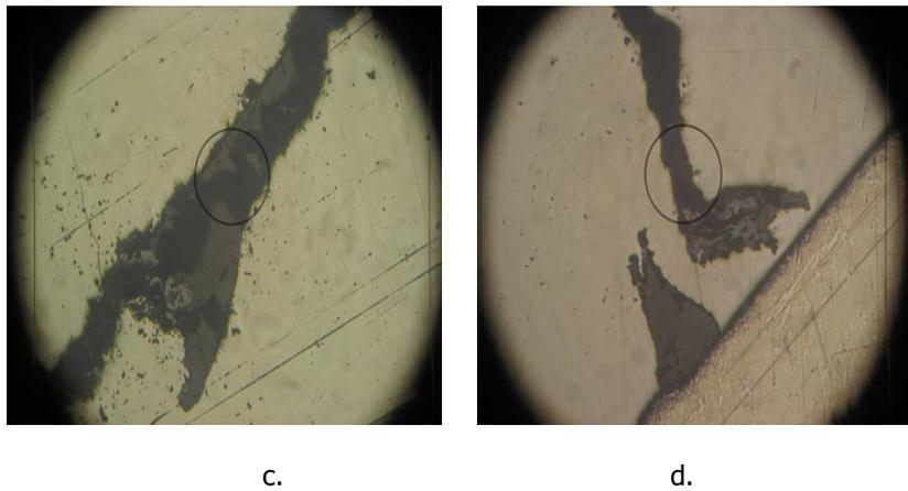
**Figure 4.** Defaults of casting in the base material (steel): a, b - bearing 1; c, d - bearing 2 (100X)
