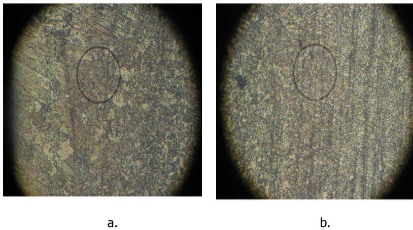
**Figure 5.** Metallographic structures of the steel stand, with pearlite-ferrite matrices – area of thermal influence: a - bearing 1; b - bearing 2 (100X)
