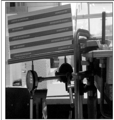
**Figure 3.** Loads on the corrugated paper board
