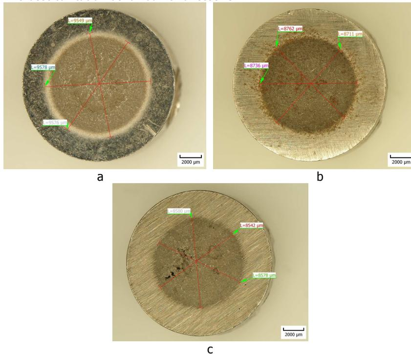
**Figure 2.** Stereomacrostructural aspect of stainless steel samples after measuring cavitation affected zone: a – steel A, b- steel B, c- steel C
